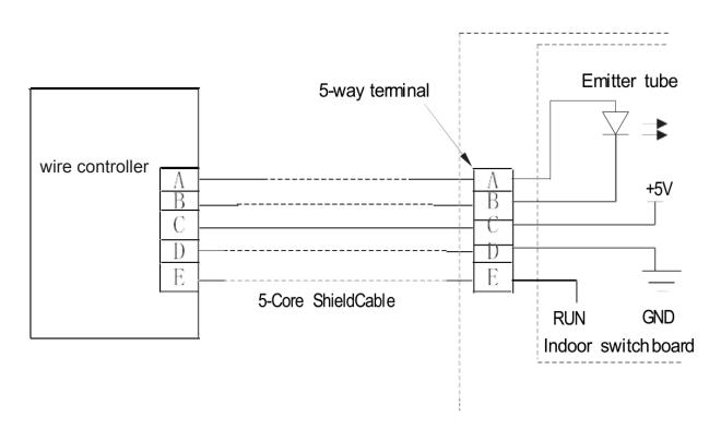
When a wire controller is needed, a small 5-way terminal should be added, fix an infrared emitter with gumwater near the receiver on the switch board. Connect its anode and cathode to A and B, and +5V, GND, RUN to C, D, E on the switch board.
